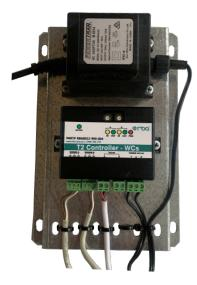
Din-plug wiring connection has been completed • in house to allow for batch test release. The unit is low voltage, 24VAC, so polarity is not critical. Ensure cable is wired to neutral and active terminals.
