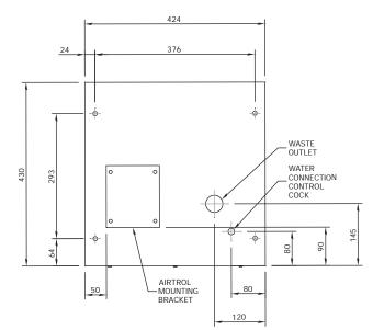
Refer to "Installation Instructions Air-Trol Valve Model 03-M" for specific valve requirements. If the Air Trol valve is to be located within the basin frame, the water supply should be terminated with a control cock as in fig. 1. Waste outlet location in fig 1 is for 40 mm plastic "P" trap. This location may vary subject to type of trap used, and should be confirmed prior to rough-in.
