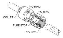
3. Pull on the fitted Tubing to ensure it is secure. Tube should not come free from the Fitting. Water test the connection assembly prior to leaving the site to ensure there are no leaks.
