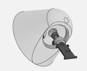
Insert the flow controller into the holder and thread into the shower body using the flat of the supplied tool. Do not overtighten.
