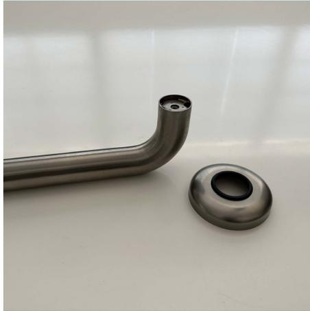
3. Slide flange cover over rail. RBA recommends adding a small amount of dishwashing liquid if the Steri+Shield™ seal is tight.
