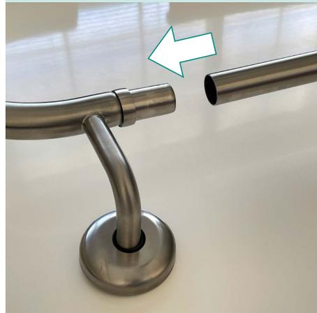
14. Slide both straight rails into place over connector piece. Please note the fixing on the connector piece is always parallel to the vertical straight rail.
