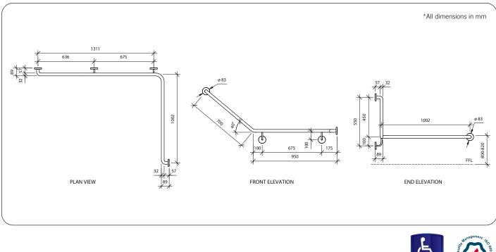
Important: Installation instructions and current rough-in details should be furnished with each fixture. Do not rough in without certified dimensions. Dimensions are subject to manufacturer's tolerance of +/-10mm.
