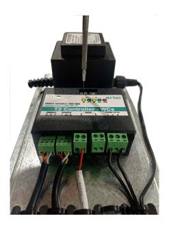
Dial A settings adjust Half Flush Timing and Dial B settings adjust Full Flush Timing.
