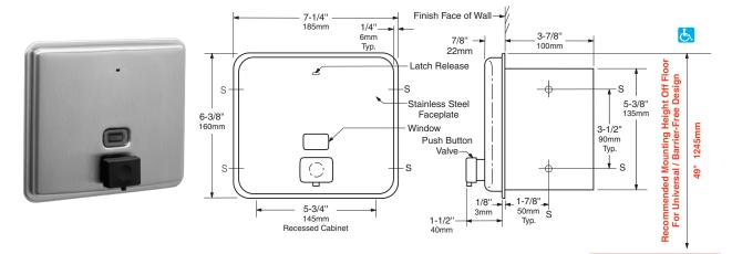
Rough Wall Opening 5-7/8" (150mm) wide 5-1/2" (140mm) high 4" (102mm) minimum recessed depth
