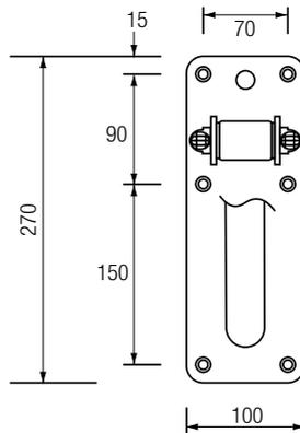
**Warning:** Grab rails are no stronger than the anchors or walls to which they are attached and must be firmly secured in order to support the loads for which they are intended.
