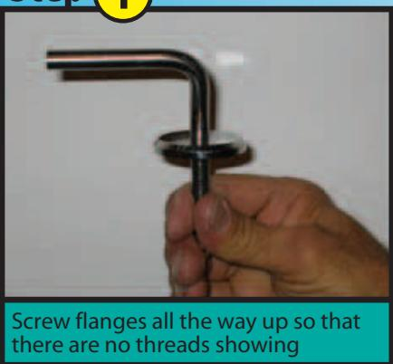
Screw flanges all the way up so that there are no threads showing
