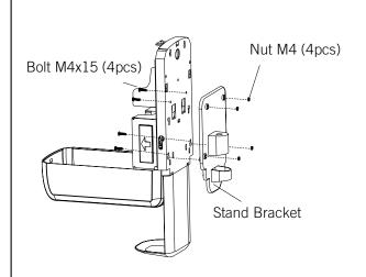
Use the 4 nuts and bolts to attach the stand bracket to the dispenser.
