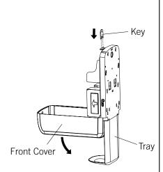
Open the dispenser with the key, then carefully remove the refillable bottle.
