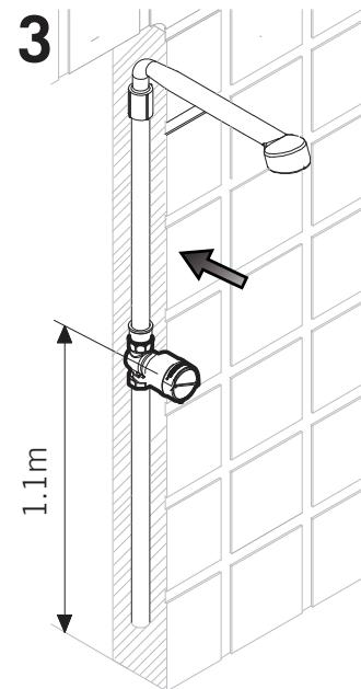
Ensure flow arrow marked on tap body aligns with intended direction of flow
